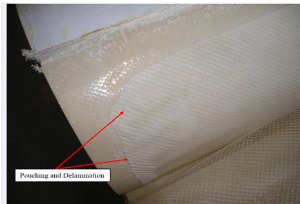
FIGURE 8 – RO MEMBRANE DELIMINATION
